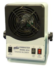
The IONMASTER® Benchtop Heated Ionizing Fan Model 6214 generates AC high voltage to produce balanced ionized airflow. It can be used either on a work surface or mounted on a wall or shelf, and directed at the work target or surface to be neutralized, eliminating static charge.
