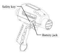
Connect the DC battery plug to the Neutralizer<sup>®</sup>AC battery jack.
