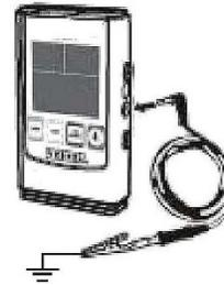
Note: for an accurate measurement, make sure the fieldmeter is connected to ground.
